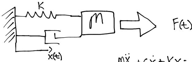
$$m\ddot{x} + cx + Kx = F(t) \rightarrow \text{no causality, just an equation}$$
